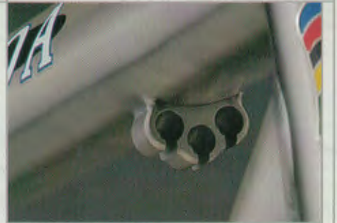
Cable routing below the top tube delivers a cleaner look along with improved cable housing intersections.
