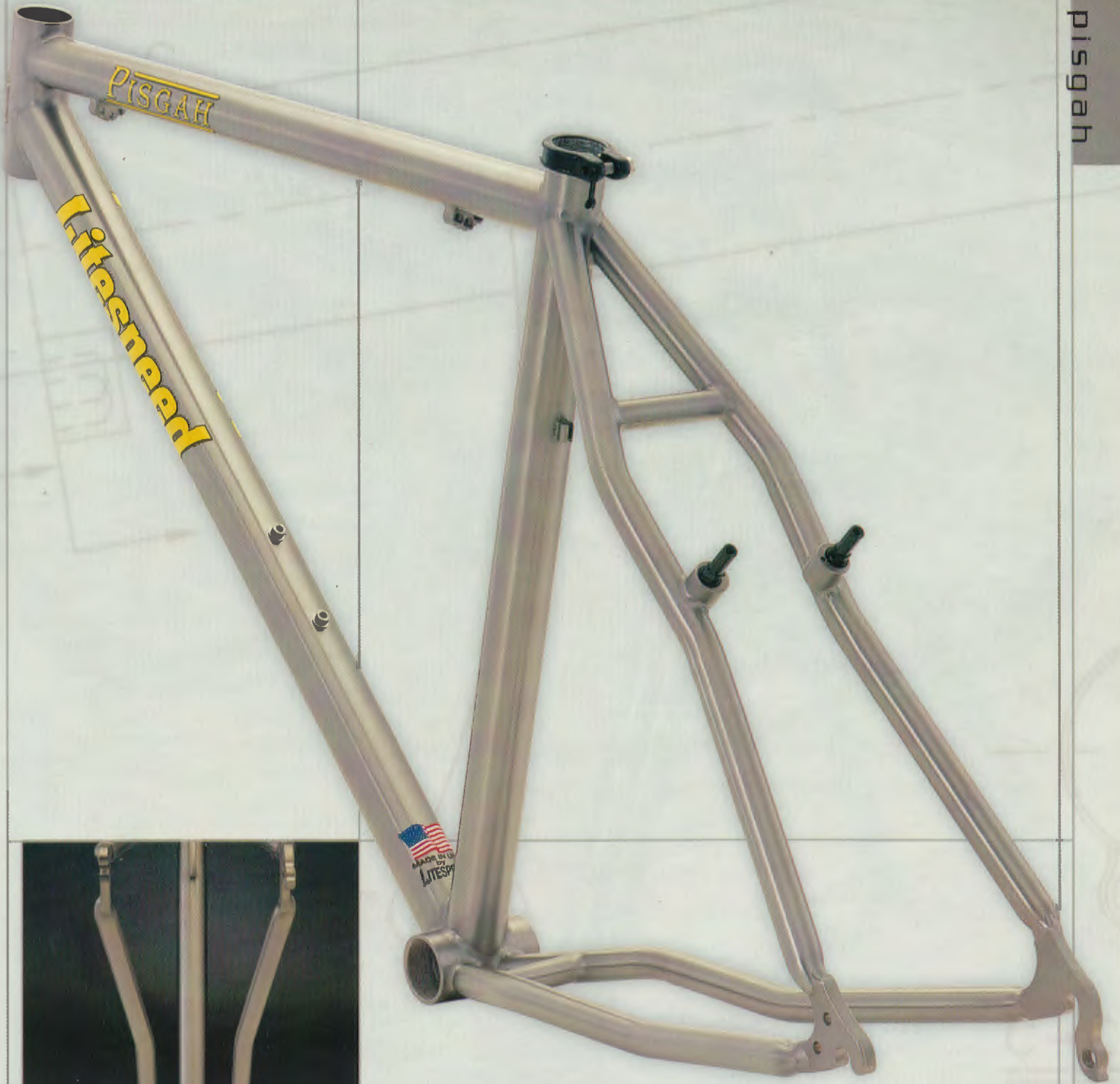
Multiplane, asymmetric chainstays add lateral stiffness, reduce chain slap, and increase crank-arm and tire clearance.
