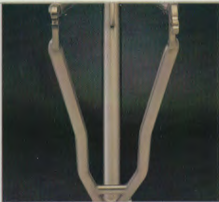
Multiplane, asymmetric chainstays add lateral stiffness, reduce chain slap, and increase crank-arm and tire clearance.
