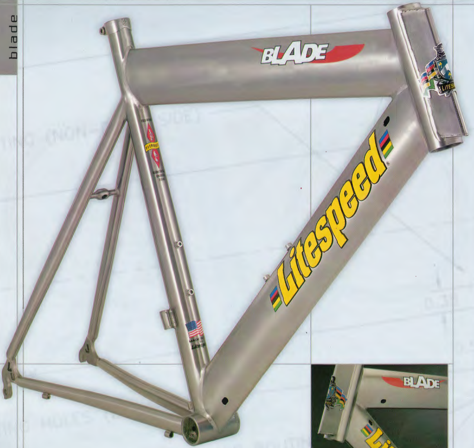
Aero-bladed 6Al-4V titanium-alloy down and top tubes combine with internal cable routing to create an extremely aerodynamic tube set.
