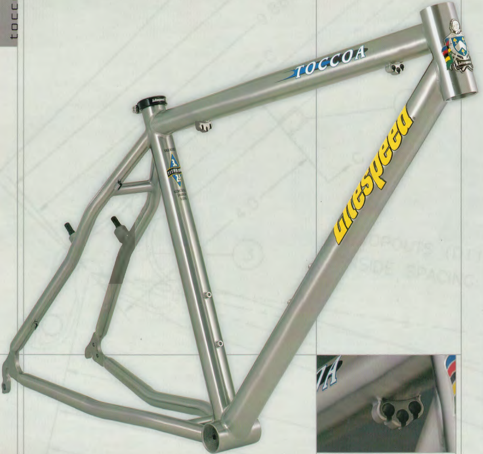
Cable routing below the top tube delivers a cleaner look along with improved cable housing intersections.
