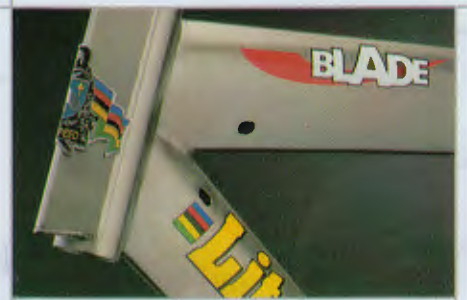
Aero-bladed 6Al-4V titanium-alloy down and top tubes combine with internal cable routing to create an extremely aerodynamic tube set.
